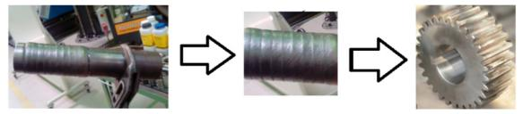
We have developed welding technology 5 different materials (Delcrome 253, 16MnCr5, 41Cr4, 50CrV4, 100Cr6) for steel C22 and analyzed the impact of parameters on the process productivity. 122 samples were welded by PTA-welding in accordance with the program, that we did, and then we cut it with a saw and
